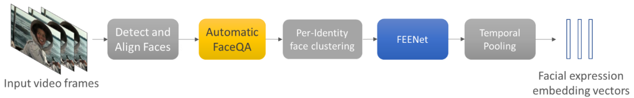
Figure 3. High-level overview of the proposed facial expression analysis pipeline for videos. First, we run face detection and subsequent automatic face quality assessment (FaceQA), which rejects faces that are blurry and/or too sideways and hence unsuited for facial analysis. Next, we cluster all faces that passed FaceQA into distinct identities. Next, we extract facial expression embeddings using the proposed FEENet, which are temporally pooled for stability.
